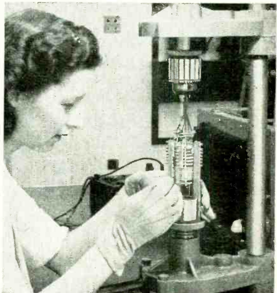
Two of the processes involved in manufacture. Optically working the flat face of the tube and (below) assembling the gun mount and electron multiplier on a jig.
